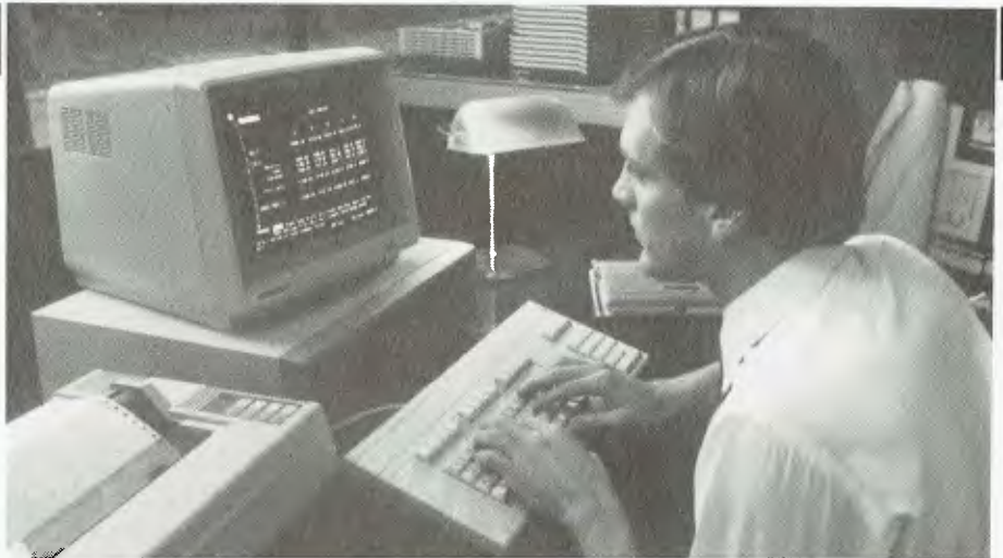
The TI Professional Computer features the innovative Speech Command System, which permits the machine to store digitised speech and recognise various words and phrases.
